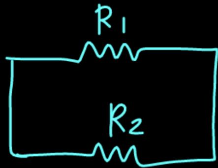
$$R_p = \frac{R_1 \cdot R_2}{R_1 + R_2}$$
